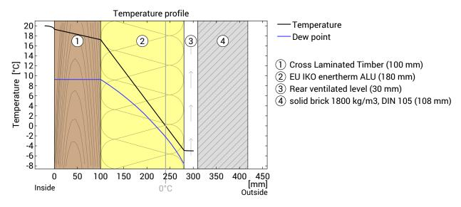
Temperature and dew-point temperature in the component. The dew-point indicates the temperature, at which water vapour condensates. As long as the temperature of the component is everywhere above the dew-point temperature, no condensation occurs. If the curves have contact, condensation occurs at the corresponding position.
