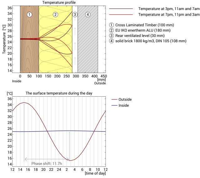
**Top:**Temperature profile within the component at different times. From top to bottom, brown lines: at 3 pm, 11 am and 7 am and red lines at 7 pm, 11 pm and 3 am.
