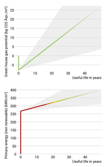
The **left figure** shows the global warming potential of the production of the component in the vertical part of the curve. Greenhouse gas emissions (through heating) arising during use of the building are indicated by the upward curve.
