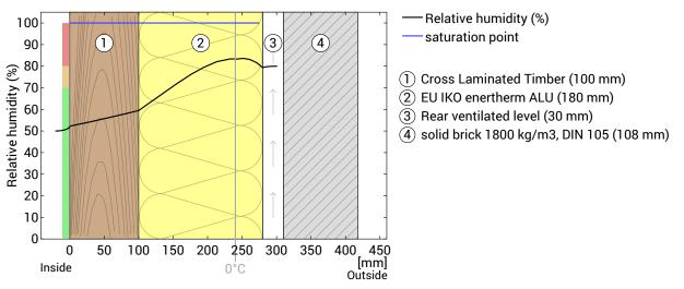
Notes: Calculation using the Ubakus 2D-FE method. Convection and the capillarity of the building materials were not considered. The drying time may take longer under unfavorable conditions (shading, damp / cool summers) than calculated here.
